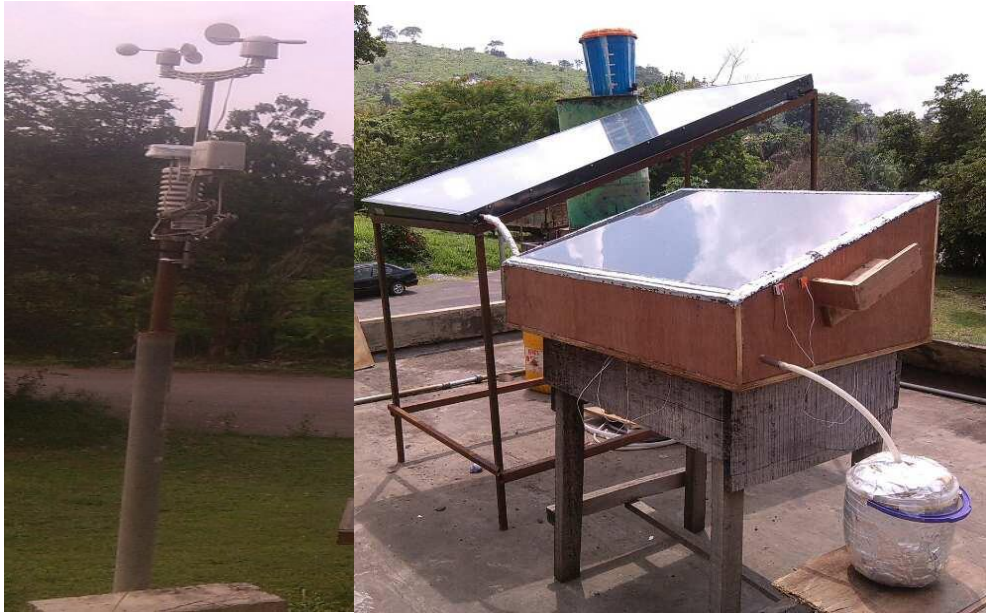
Figure 2: Experimental set up of solar still coupled with flat plate collector
