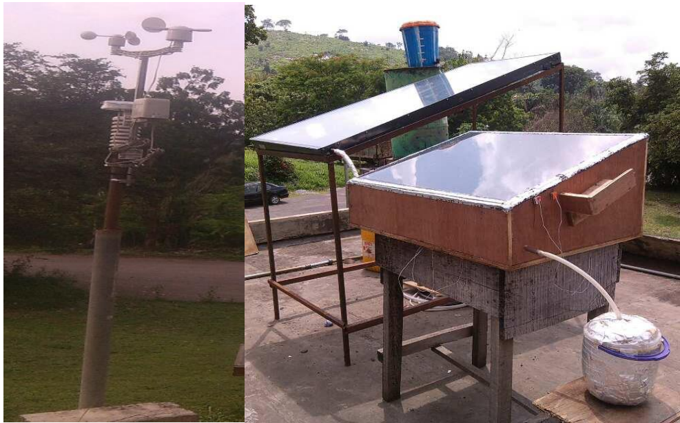
Figure 2: Experimental set up of solar still coupled with flat plate collector
