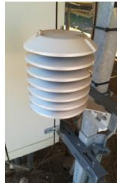
51 Ambient temperature sensor
