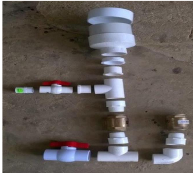
Fig. 2 Picture of pump components
