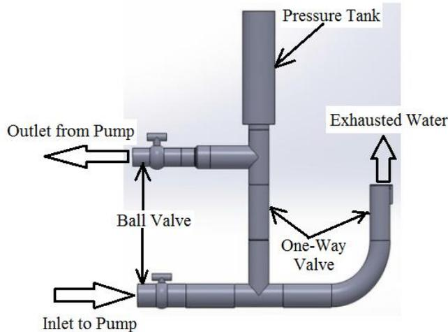
90 **Fig. 1** Schematic of Hammer Head Pump
