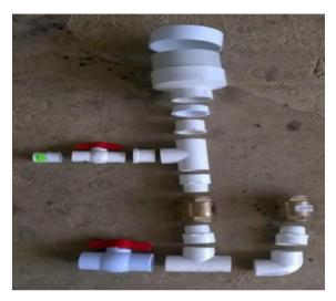
Fig. 1 Schematic of Hammer Head Pump
