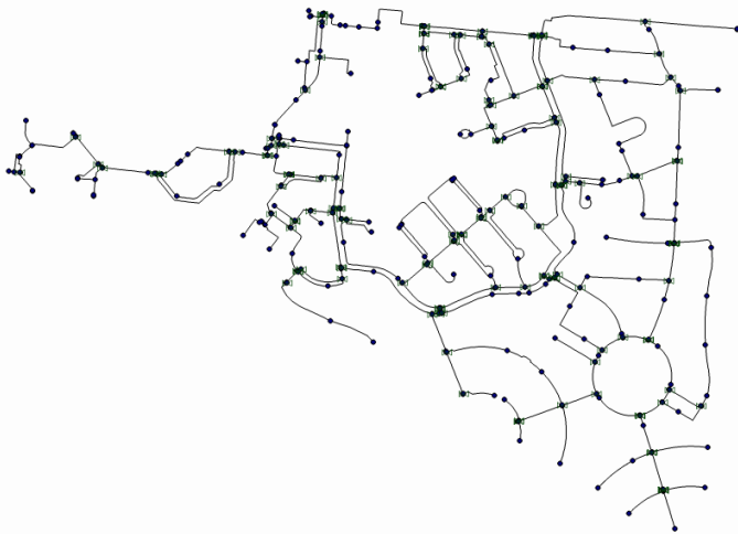
15 Figure 1: EPANET model of the drinking water distribution network of Sittard (Netherlands), consisting of 584-583 nodes/junctions , 491 links-pipes , 140 valves and 1 reservoir.
