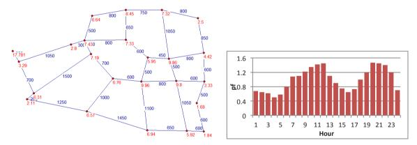
Fig 4. (a) Layout of Safi town network (including nodal base demands and pipes lengths); (b) Domestic demand pattern.
