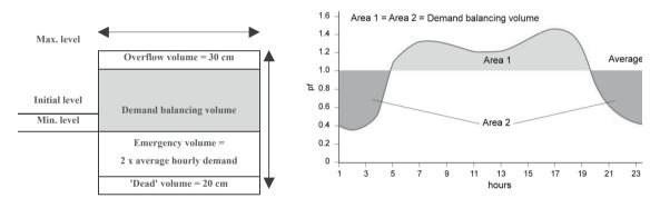
Fig. 1. (a) Required tank volume; (b) Demand balancing volume (adapted from Trifunović, 2006)
