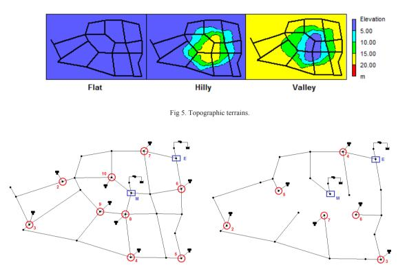
Fig 6. (a) Looped scheme with source and tank locations; (b) Branched scheme with source and tank locations.
