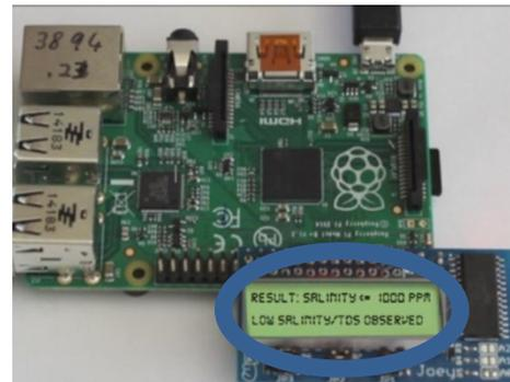
**Fig. 7 (a) Integrated Device display with Raspberry Pi (red circle), (b) 2000 ppm salinity result (yellow circle) (c) 1000 ppm salinity water result (blue circle)**
