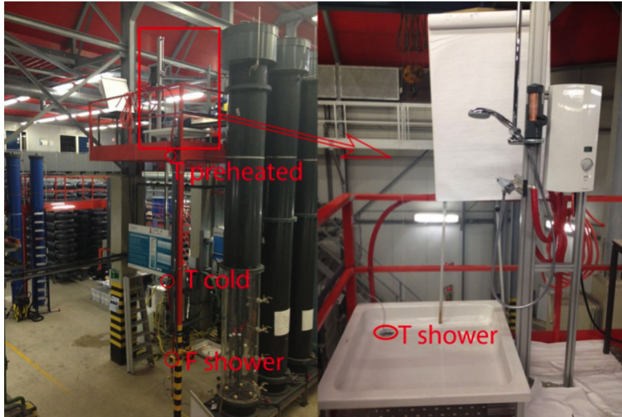
Figure 3. Experimental setup of the laboratory configuration.
