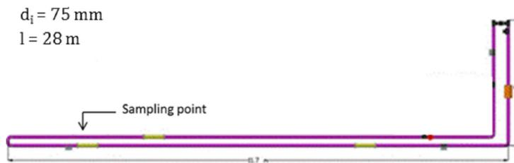
**Fig. 1.** Illustration of the pilot loop used.
