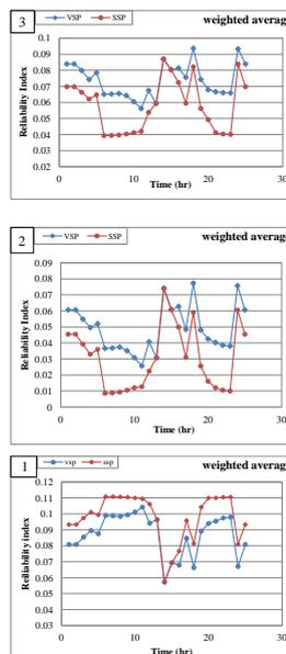
**Fig. 1.** The comparison of reliability of two type of pumps (VSP, SSP), with weighted average of four scenarios using three nodal pressure equations.
