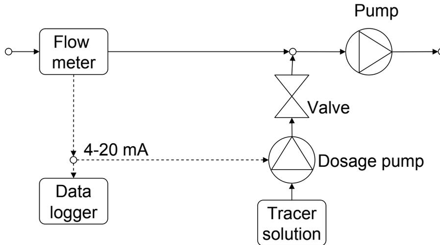
**Fig. 2.** Measurement setup for adding tracer solution.
