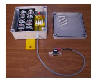
Fig. 2. Small-sized accumulative water meter.
