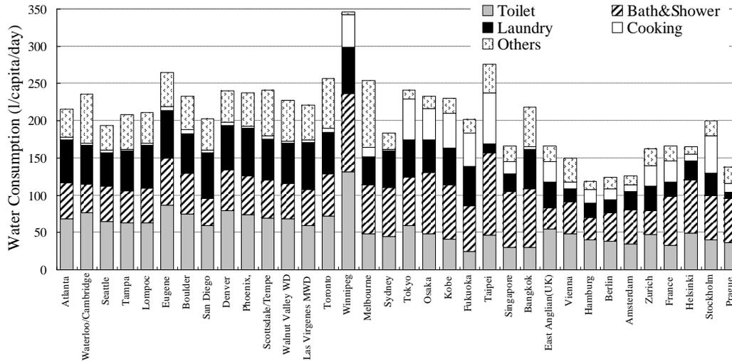
**Fig. 1.** Micro-components of residential indoor use.
