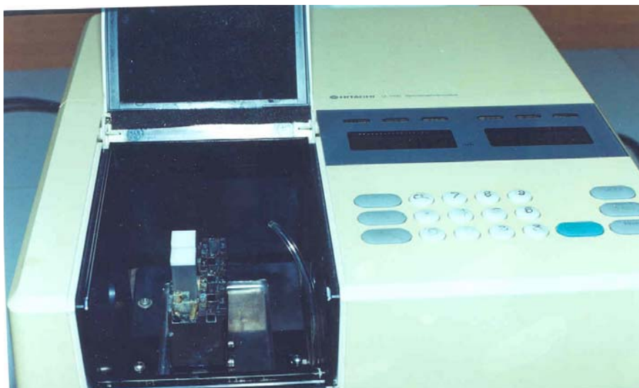
Fig. 2. Suction system to rectify fogging problem.
