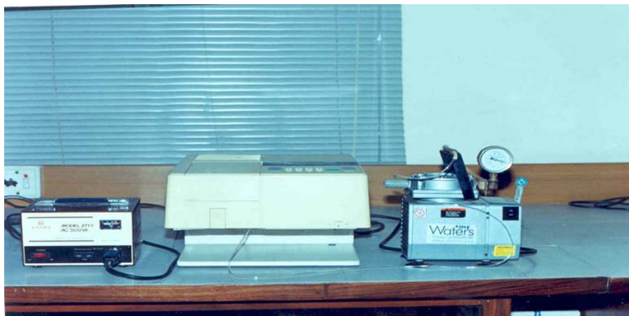
Fig. 3. Suction system to rectify fogging problem and stabilizer to control voltage variation.
