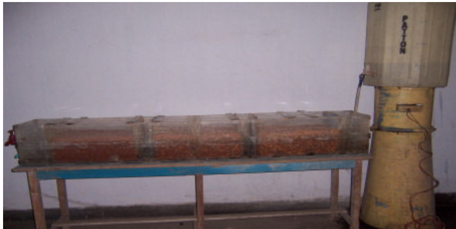
Fig. 1. Model of horizontal roughing filter used in the experiment.
