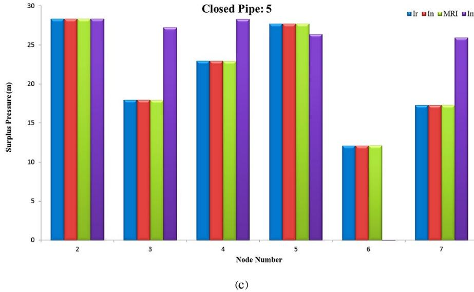
Fig S1. Surplus pressure of nodes in two-loop network for solution with maximum reliability criteria under failure of pipes No. (a) 2, (b) 3 and (c) 5
